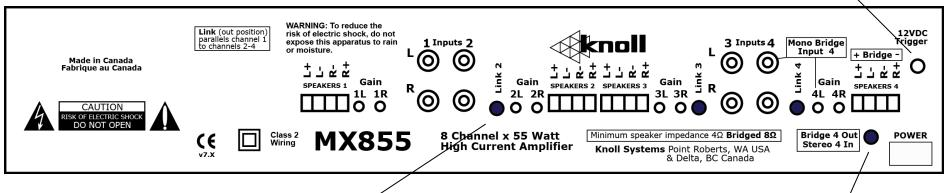
The Link button is normally set to the "in" position to give all six stereo inputs individual sources. When the Link button is set to the "out" position, that input Left/Right is linked or cascaded (or paralleled) to input #1 (without the use of Y cords). Any or all combination of linked inputs 2 to inputs 4 are possible. When all inputs are linked to input 1 the input impedance is about 6000  $\Omega$ .
